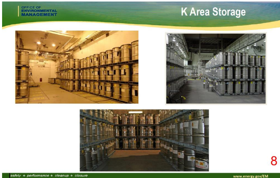
photos: Storage in the K Area Facility at SRS of "9975" storage containers holding weapon-grade plutonium in "3013" cans; in presentation to SRS Citizens Advisory Board, July 28, 2015
